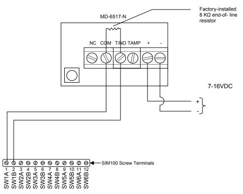
Figure 1 – Wiring Diagram
